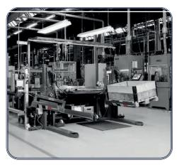
The tilt function reduces the reach distance for the operator. The forks can be tilted up to 40 degrees (both left and right).
